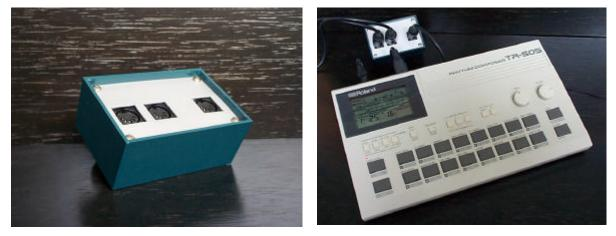
With the ESI<sup>TM</sup> syncbox you can convert midi standard timing signals to roland<sup>TM</sup> sync24. Now you can sync your Roland<sup>TM</sup> MC202, TB303, TR606 and TR808 with your midi setup. You can sync with your computer program for studio use or with a midi drumcomputer (e.q. a TR505) for live performance.
